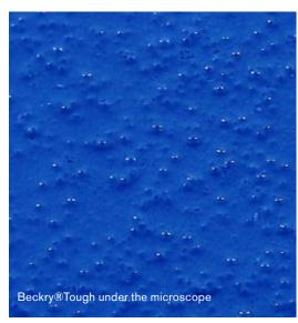
By varying the type, particle-size and dosage of polymeric beads, the visual effects become almost unlimited.
