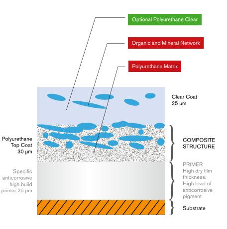
Beckry®Tex PUR is a topcoat based on polyurethane resin that offers a very high outdoor durability and makes it possible to achieve high dry film thickness. It gets a textured surface when cured and contains polyamide giving the surface a very good scratch and wear resistance. Beckry®Tex PUR has excellent colour and gloss retention as well as chemical resistance. It is recommended to be used in conjunction with the high build polyurethane primer Beckry®Prim.
