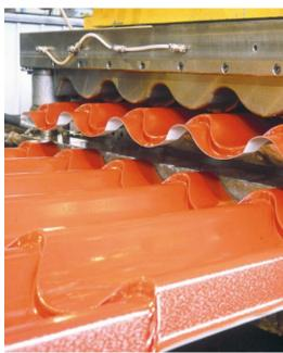
Beckry®Tough derives its surface texture from the incorporation of polymeric beads in the paint formulation.
